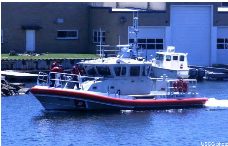
Station Oswego asset: 45-foot RB-M (Response Boat-Medium).
