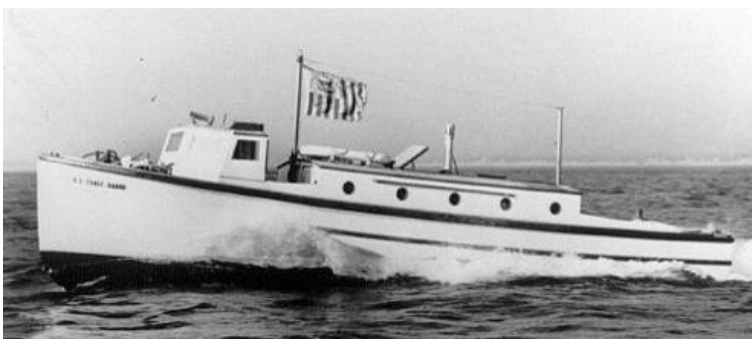
38-foot Picket boat: Self-bailing but not self-righting; 38ft. 3in. overall length, 10ft. 5in. beam, 3ft. maximum draft; 16500lbs.; single gasoline engine of various makes and models with single propeller; maximum speed 24-25kts.; 240gal. fuel; 175 nautical mile range at cruise speed; capacity for 2 crew plus 10 passengers; wooden hull of single-planked carvel construction; hull was ice-sheathed if intended for assignment to an area where ice could be encountered.
