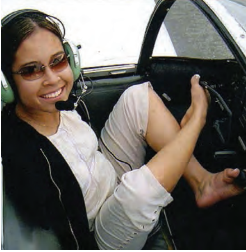
Jessica demonstrates how she flies her 1946 Ercoupe airplane. Left foot on the throttle, right foot on the yoke, for steering.
